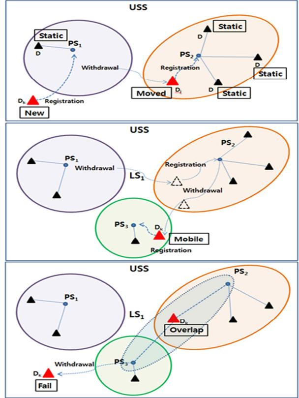
Figure 3. Device Status Types for Device Management: NEW, STATIC, MOVED, OVERLAP, MOBILE, FAIL.
